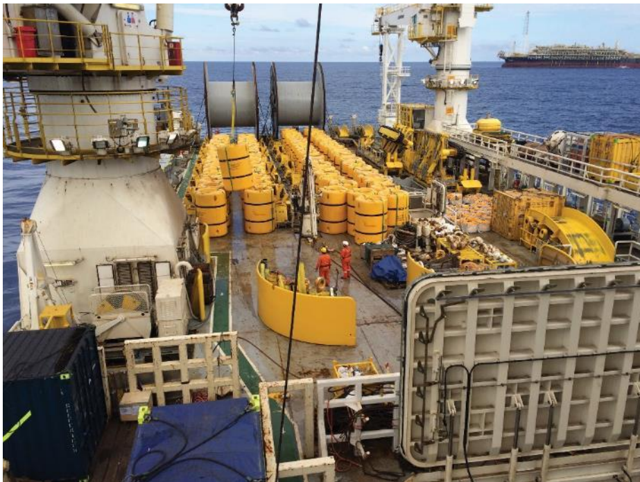
Figure 22 Buoyancy modules stored on a vessel prior to installation. Image courtesy of Balmoral. All rights reserved.
