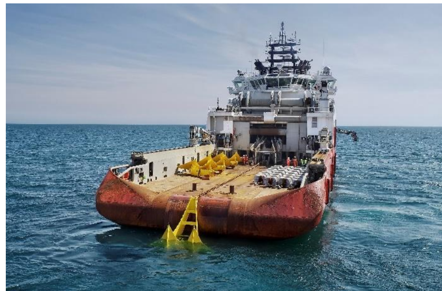
Figure 39 Anchor-handling vessel. Image courtesy of Vryhof. All rights reserved.
