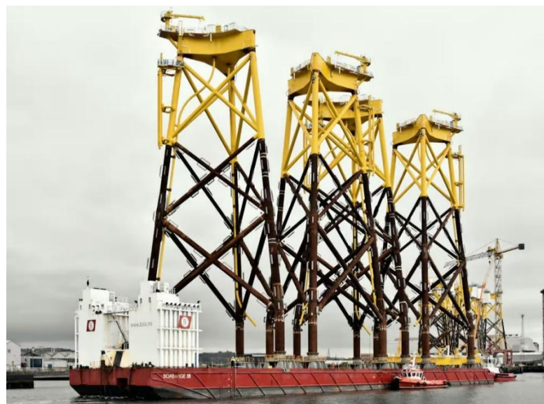
Figure 11 Example of jacket foundations being transported.
