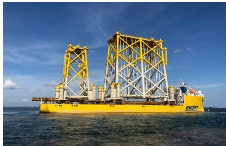
Figure 33 Offshore substation jackets. Image courtesy of Ørsted. All rights reserved.
