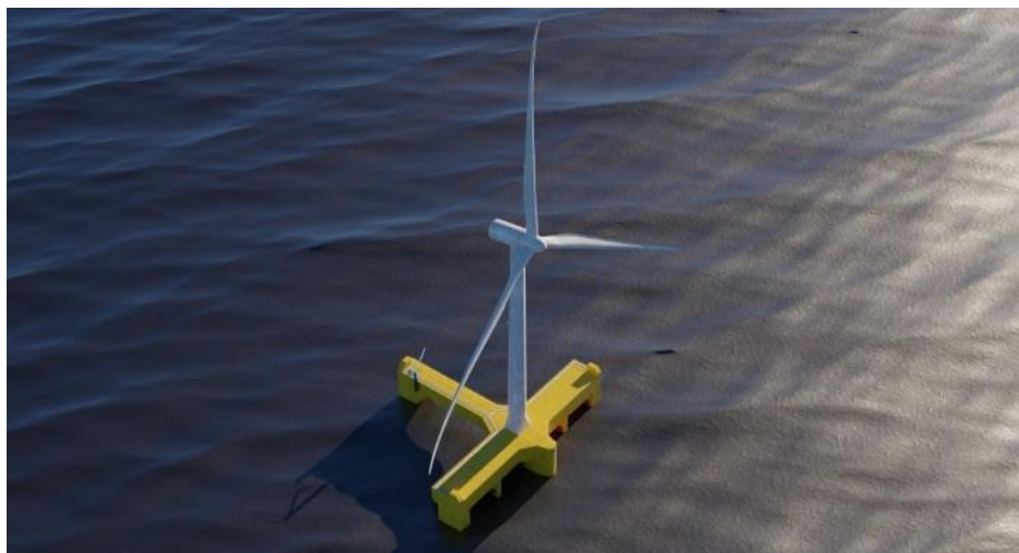
Figure 9 Combined wind and wave device. Floating Power Plant's substructure (image courtesy of Floating Power Plant, all rights reserved).
