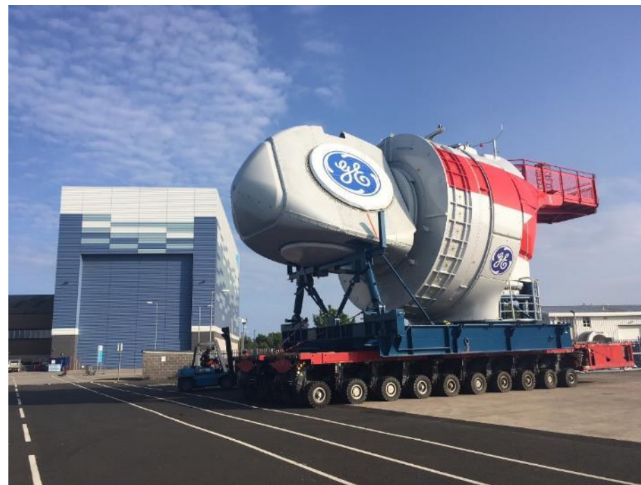
Figure 14 GE's Haliade X 12 MW nacelle. Image courtesy of GE Renewable Energy. All rights reserved.
