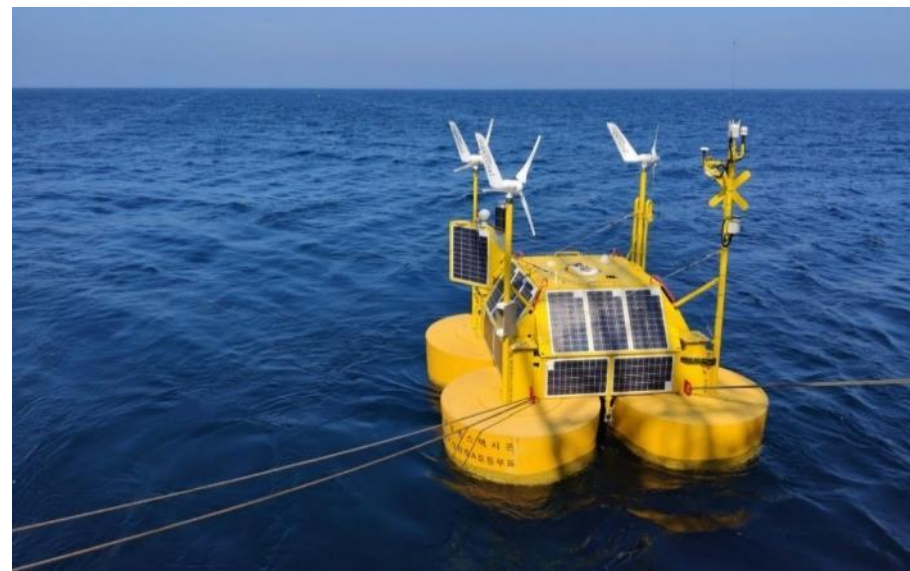
Figure 12 Example of a floating lidar used to capture atmospheric data. Image courtesy of EOLOS. All rights reserved.
