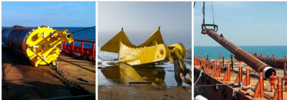
Figure 29 Suction pile anchor, drag embedment anchor and driven pile anchor. Images courtesy of Acteon, Principle Power and Acteon. All rights reserved.
