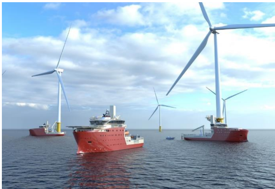
Figure 48 Fleet of service operation vessels servicing a fixed offshore wind farm. Image courtesy of North Star Renewables. All rights reserved.
