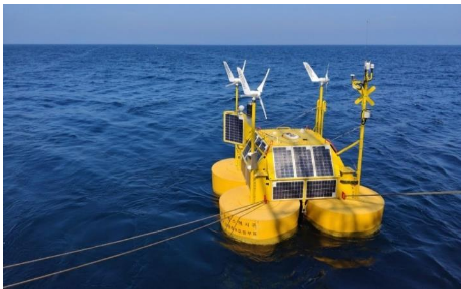
Figure 10 Example of a floating lidar used to capture atmospheric data. Image courtesy of EOLOS. All rights reserved.
