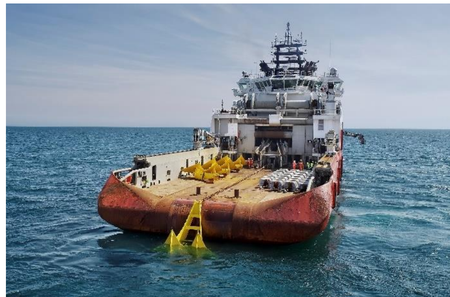
Figure 37 Anchor-handling vessel. Image courtesy of Vryhof. All rights reserved.
