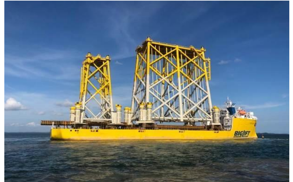
Figure 31 Offshore substation jackets. Image courtesy of Ørsted. All rights reserved.
