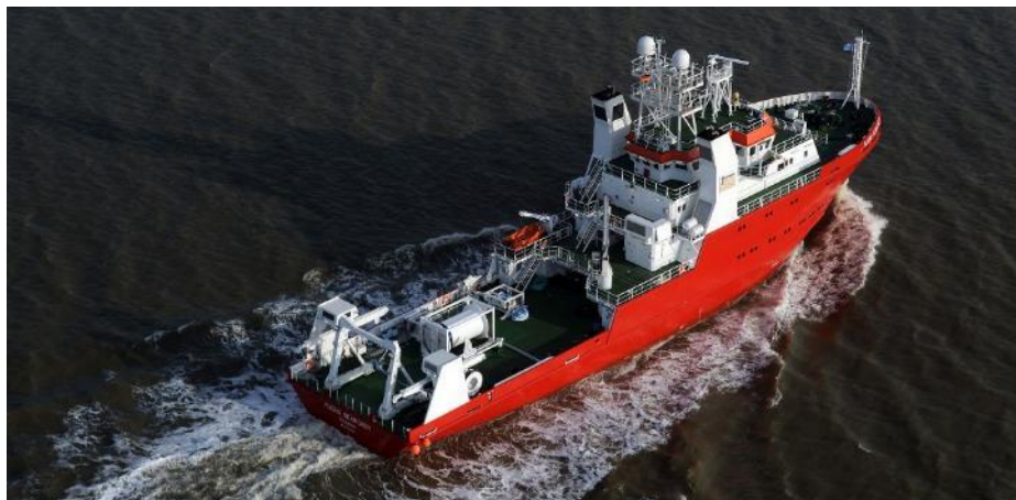
Figure 11 A specialist geophysical survey vessel. Image courtesy of Fugro. All rights reserved.
