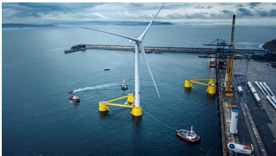
Figure 41 An assembled floating offshore wind turbine starting its tow-out for the WindFloat Atlantic project. Photo of the WindFloat Atlantic project courtesy of Principle Power/Ocean Winds.
