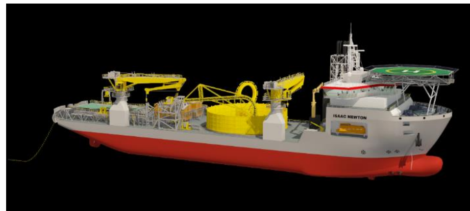
Figure 35 Cable-laying vessel. Image courtesy of Jan de Nul. All rights reserved.
