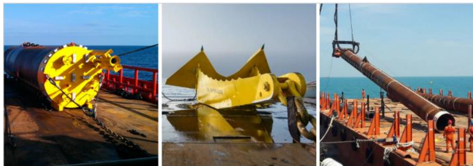
Figure 27 Suction pile anchor, drag embedment anchor and driven pile anchor. Images courtesy of Acteon, Principle Power and Acteon. All rights reserved.
