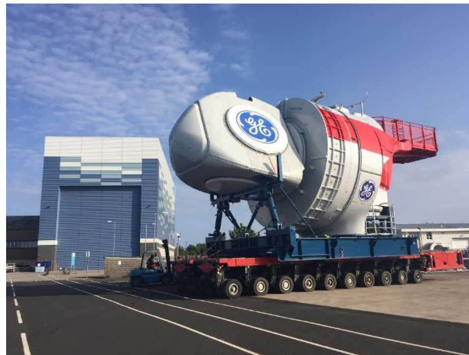
Figure 12 GE's Haliade X 12 MW nacelle. Image courtesy of GE Renewable Energy. All rights reserved.
